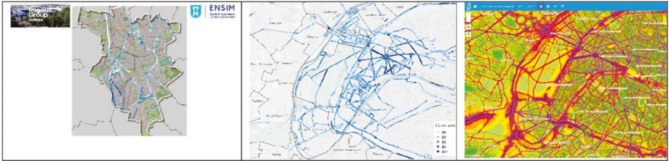
Example of mapping generated from APACHE data and simulation results from Bruitparif.
