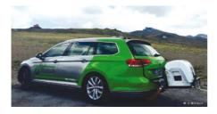
**V-Motech** has set-up a specific competence cluster dedicated in exhaust measurement and analysis to perform RDE LDV tests. V-Motech's technical skills completes the PEMS technology which allows the concentration measurement of five gases while adding and Exhaust Flow Meter (Pitot tube device) and an ODB system to obtain the vehicle diagnostics.
