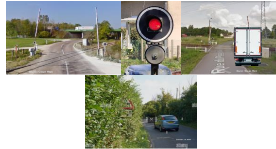
Figures 5 to 8: Illustration of SOTIF triggering conditions in level crossing areas (from left to right) [4]: Rail tracks with high contrast compared to the pavement, R24 traffic light, Parked vehicle masking R24 traffic light & barrier, Vegetation masking the traffic sign
