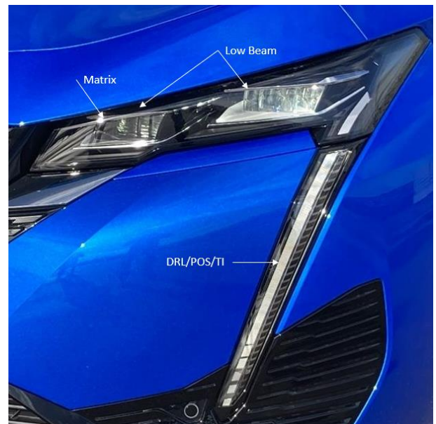
Figure 2: 308/408 front face – upper version
