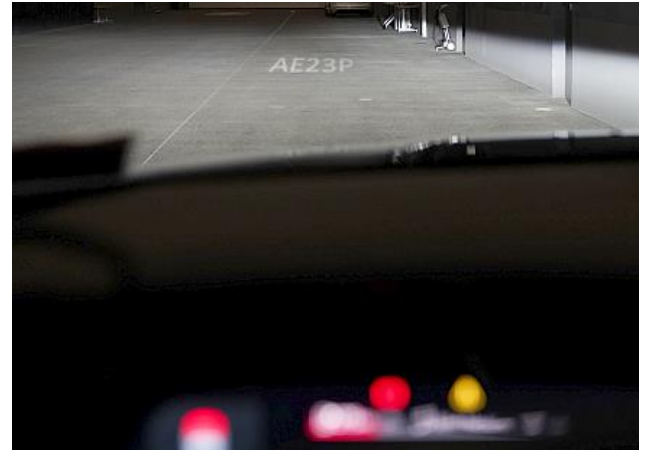
Figure 6: Example of Readability Pattern "AE23P" used in the investigation from driver's perspective (20 .. 24m)
