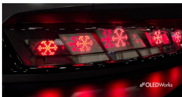
Figure 3: Demonstration OLED Rear Combination Light Displaying Snow Hazard Information
