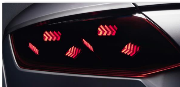
Figure 4: OLED Panels with Over 200 Segments per Panel and 3-15 mm 2 Segments
