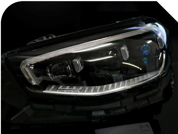
Figure 1: Smart Corner Prototype - Head Light with integrated LiDAR Module
