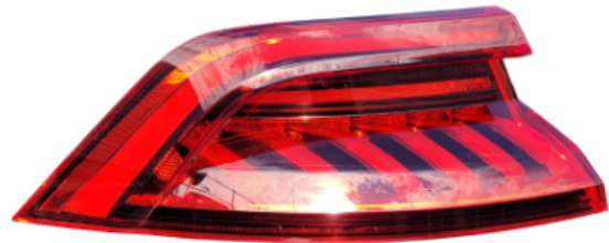
Figure 16: Phantom effect on Rear Lamp
