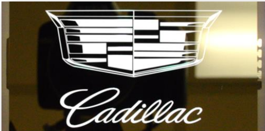
Figure 9: Example Badge OLED Panel
