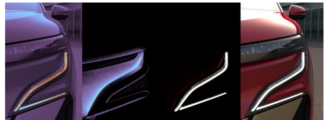
Figure 3: Objective evaluation for homogeneity, leak of light analysis, design validation.
