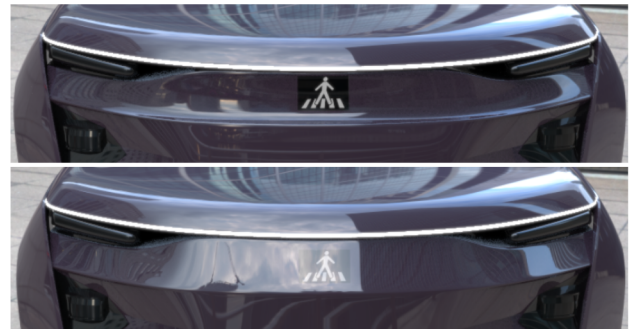
Figure 18: Impact of the outer lens inclination on contrast and required Brightness
