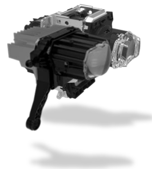
Figure 9: Illustration of a LED-ADB High system by a module combination of a bi-function LB/ADB 1-row and a HD-projection module
