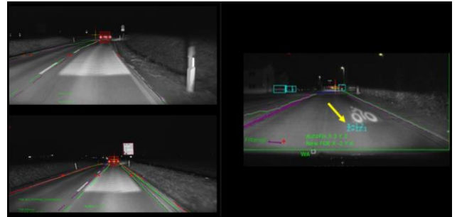
Figure 8: Camera recognized shapes of projecting headlights
