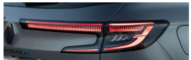
Figure 3: Moiré effect on Austral rear lamp
