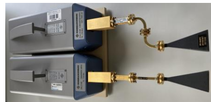
Figure 1 - Details of the quasi-monostatic configuration for the antenna with the connecting elbows
