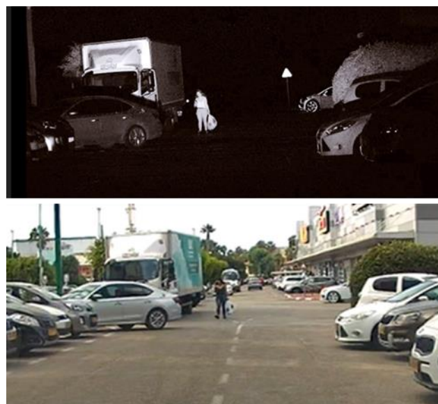
Figure 4 – Range discrimination as a detection enhancer (GatedVision - top)
