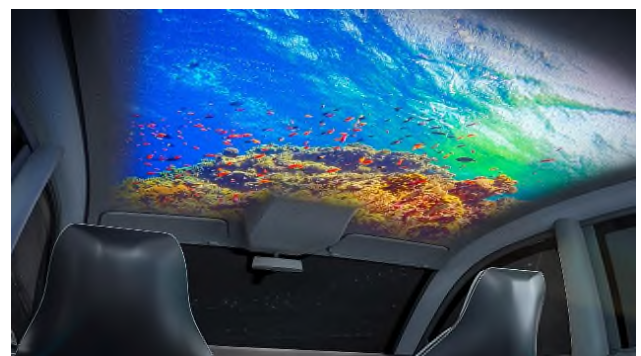
Figure 5: Headliner projection application for widescreen display of animations over multiple materials and structures
