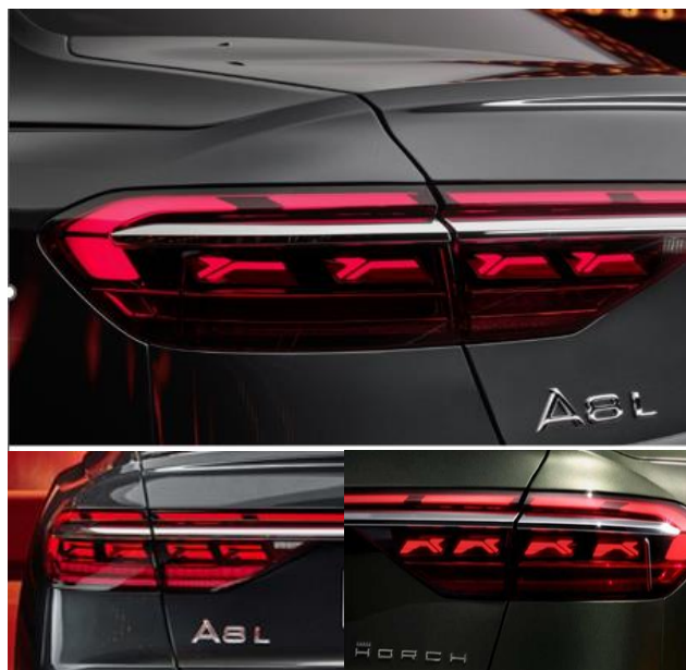
Figure 2: Audi A8 OLED Taillights with Personalized Tail Position Signatures
