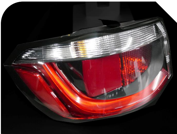
Figure 2: Smart Corner Prototype - Rear Lamp with integrated RADAR Module
