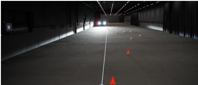
Figure 18: Average Readability Zone marked in the light tunnel with pylons. Oncoming Situation.
