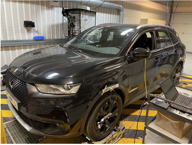
Fig. 1: DS Automobiles DS7 prototype car on the four-post test rig
