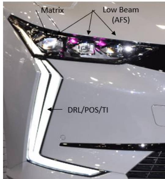
Figure 1 : DS4 Front face upper version
