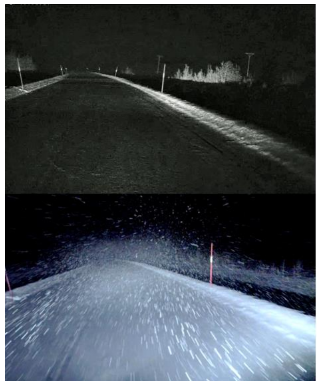
Figure 5 - Backscatter in snow. GatedVision (top) vs. a visible HDR camera (bottom).
