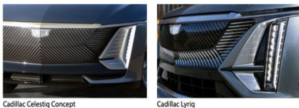
Figure 2: Arrangement of lighting modules in vertical lines, Source: DVN-Report [1].
