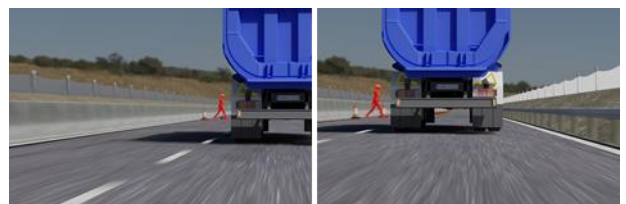
Figure 4: FOV Rendering - Head Lights (left) vs. Roof Mount (right)
