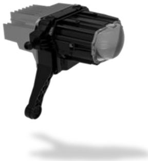
Figure 7: Illustration of a LED-ADB Entry LB/ADB 1-row projection module
