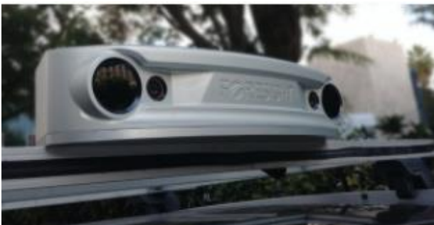
Figure 4: QuadSight vision system by Foresight 2
