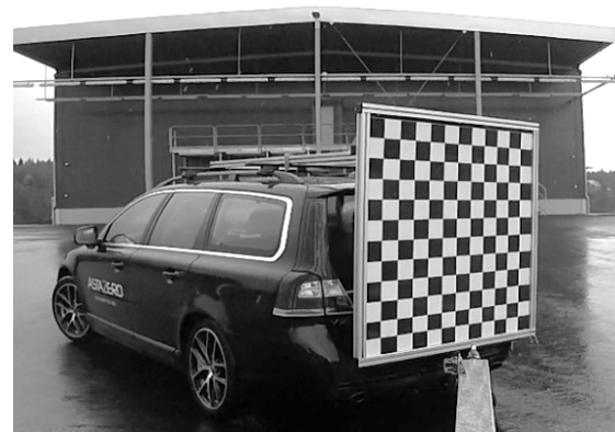
Figure 1 Checkerboard contrast target mounted on a Volvo V70
